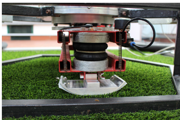
Figure 35: test foot in position having the load applied
