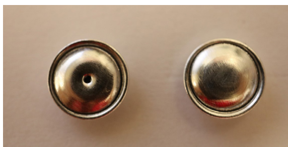
Figure 52: vented crucible (left) and unvented crucible (right)
