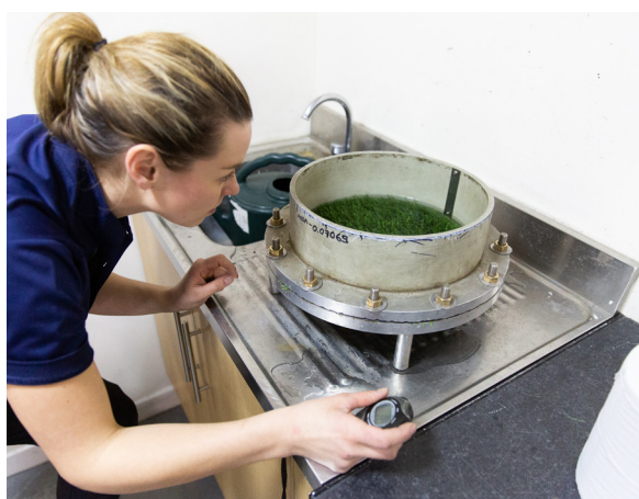
Figure 55: example of apparatus for porosity testing
