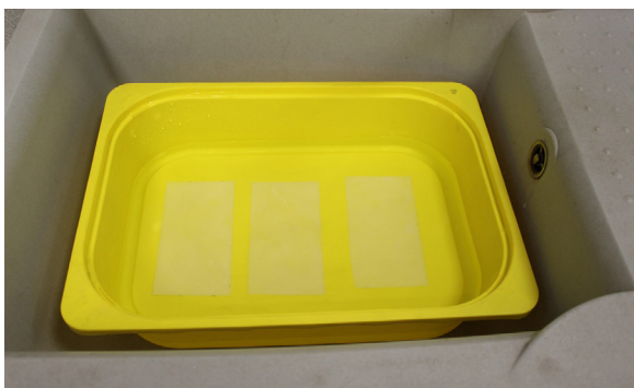
Figure 23: skins immersed in water with smooth surface facing upwards
