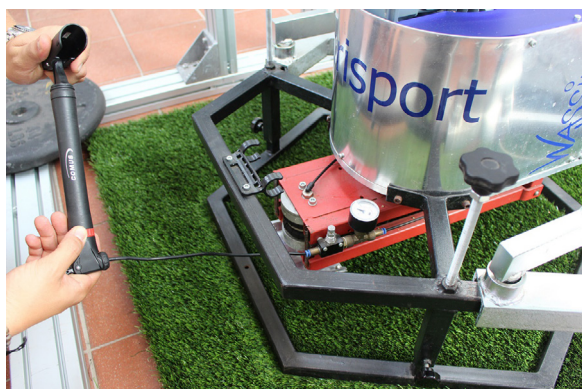
Figure 35: test foot in position having the load applied
