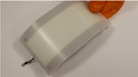
Figure 29: test foot with silicon skin taped
