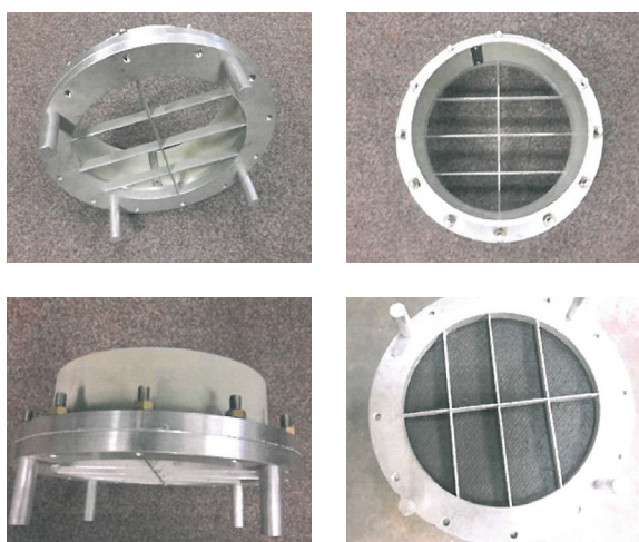
Figure 55: example of apparatus for porosity testing
